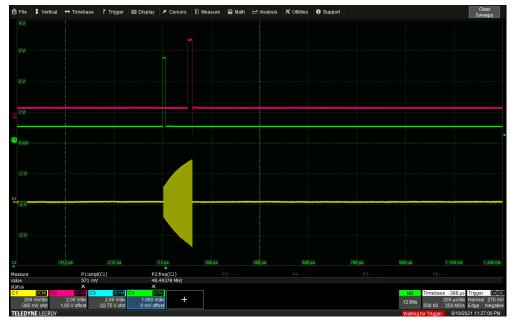
EXT trigger, Pulses #(n+2)....#(n+12) = Trigger each Image3 repeat (11off). Same scope plot as above.
